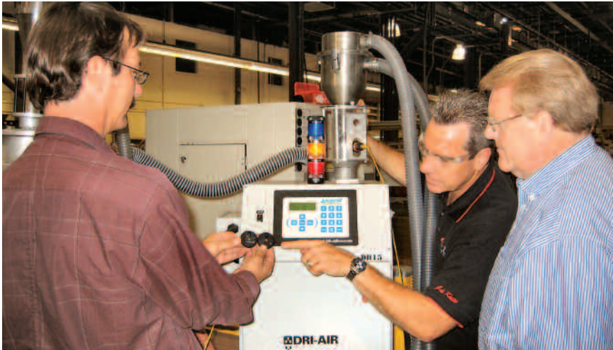
The precise metering capabilities of its dryers allow Toro to simply dial in the concentrate percentage required for its laser-etched components.
