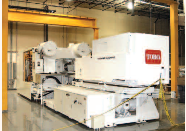
A brand-new 1450-ton, twin-platen Toshiba is a recent addition to Toro El Paso's press capacity.
