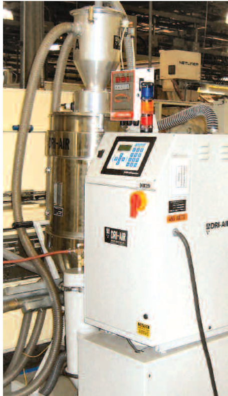
A closed-loop, Dri-Air H Series four-bed dryer precisely and repeatedly dries TPU filled with a special concentrate that allows Toro to laser-etch precision molded sprinkler components. Toro was so pleased with the dryer's performance it bought 30-plus more.
